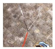
The pot can be threaded back through the f-hole to its mount
