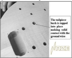
Installing the tailpiece bushing may be done with a plastic headed mallet or place a small piece of wood on top of the bushing to prevent damage and top the bushing in place with an ordinary hammer. Now screw the tailpiece mounting screws back into the bushings.
