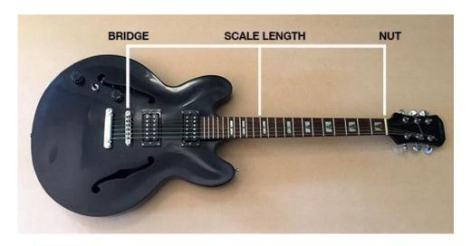
If you are working on a set neck (glued-in neck) put the neck in place and then grab a tape measure or ruler and measure from the inside of the nut to your 12th fret. When the neck is correctly in place the distance from the inside of the nut to your bridge saddles should be double this measurement. Make sure you get this right and then mark the back of the neck with a straight line to ensure you have the positioning perfect when you glue the neck in place.
